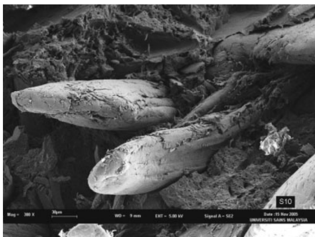
Figure 3 Fracture surface of composite with EFB pulp prepared from 10% NaOH soda pulping.
